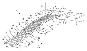
Like the Distinguishing Guise, this patent describes a ramp which includes a pair of parallel rails being connected by bars which define the ramp surface and rubber coated fingers which grip the truck gate. Also like the Distinguishing Guise, the patent describes that the ramp can be shipped as a kit of small parts and assembled by consumers using conventional tools.
