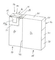
Pack made of thin cardboard, especially for cigarettes. In slide packs, a cigarette group (11) enwrapped by an inner wrapping (12) is located within a box part (17) being open at the top. This box part (17) is slideably arranged in a casing (18) open on one side (push-out opening 29). An oppositely situated side wall (30) is closed except for an
